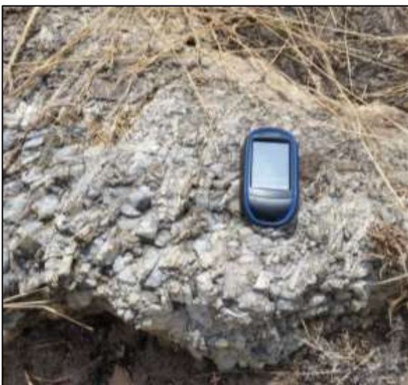
Coarse grained "crowded" spodumene rock at Goulamina
